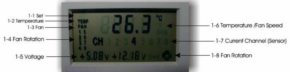
Fig.1 LCD Display (Back-light Off)
