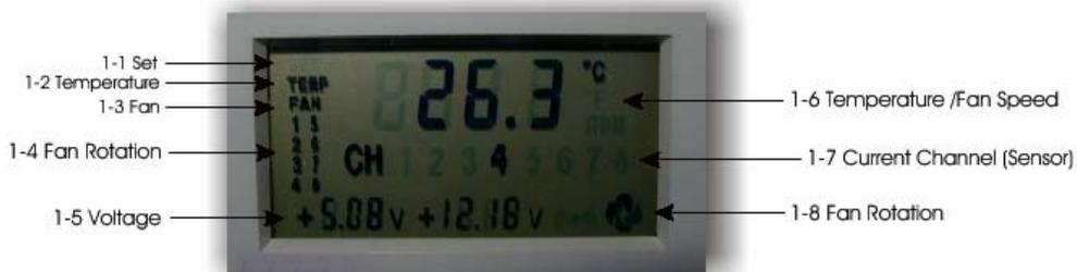
Fig.1 LCD Display (Back-light Off) - Normal Operating Mode
