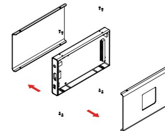
b) Install the hard drive and mount it with the two screws from the bottom through the frame and circuit board. Replace the covers and fasten the screws to finish the assembly.
