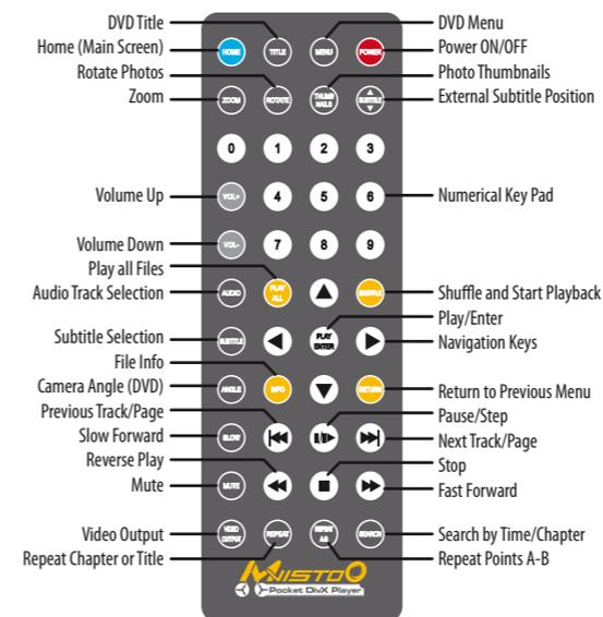
Note: Pressing the Video Output button does not save the video output. To confirm a change, go to Video Settings in the Settings menu, select the corresponding output and press the Home key to save the new setting.
