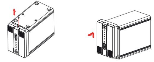
b) Install the hard drives as illustrated below with the top of the drives, where the label is located, facing each other. Push the drives lightly into place and then replace the front panel. Mount the front panel and the drives by fastening the screws at the bottom of the case.
