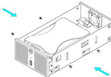
7. Slide the inner enclosure back into the outer chassis.
