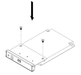
4. Slide the bridge board and hard drive back into the enclosure.
