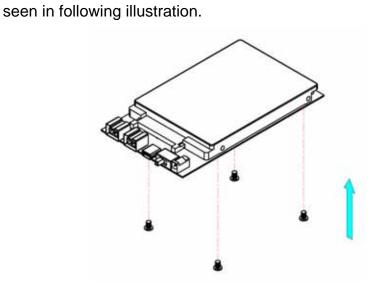
4. Mount the hard drive with the four screws from the bottom as
