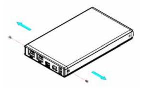
2. Remove the rear panel and pull the bridge board gently out of the enclosure.
