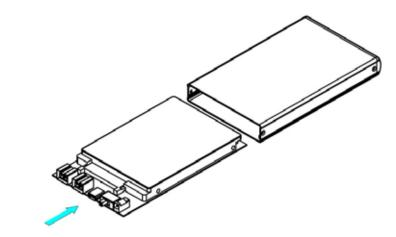
6. Fasten the two screws for the back panel to finish the assembly.
