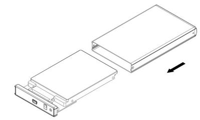
5. Fasten the two screws for the back panel to finish the assembly.
