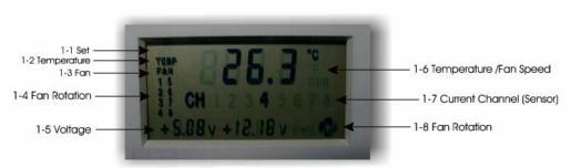
Fig.1 LCD Display (Back-light Off) - Normal Operating Mode
