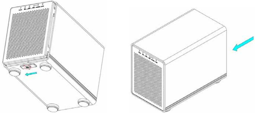
2. Pull the front panel out and then lift it up to remove it.
