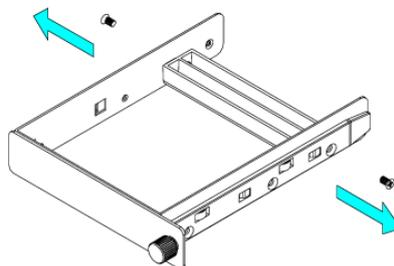
5. Install the hard drive as illustrated below with the SATA connector facing away from the front.
