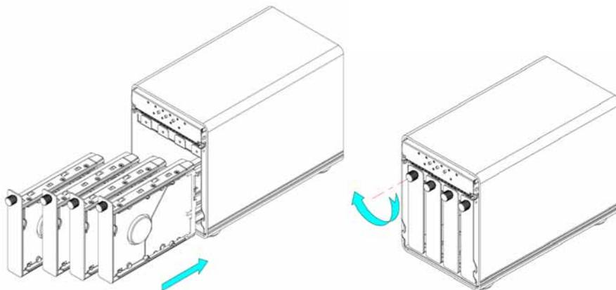
9. Align the bottom of the front panel with the notch in the chassis and then push it lightly into place.
