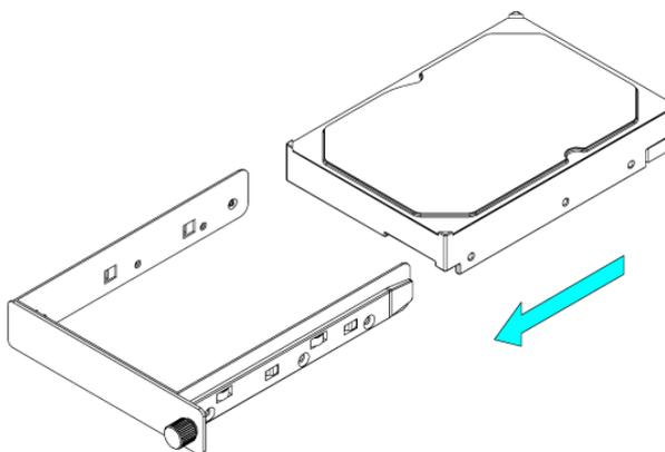
6. Mount the drive with the six screws from the side.
