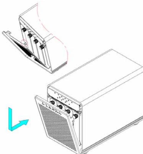
10. Unlock the switch at the bottom of the case and then push the inner chassis back into the housing.
