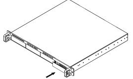
2. Install the hard drive as illustrated below with the SATA connector facing away from the front. Mount the drive with the four screws from the bottom.
