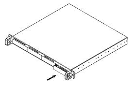
2. Install the hard drive as illustrated below with the SATA connector facing away from the front. Mount the drive with the four screws from the bottom.
