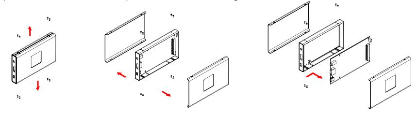
b) Install your hard drive but be careful not to damage any pins or components! Jumper settings of your hard drive should be set to Master. Fasten the hard drive to the frame and bridge board with the two (2) screws. Replace the covers and fasten the screws.
