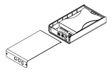
6. Fasten the 2 screws on the rear panel to finish the assembly.
