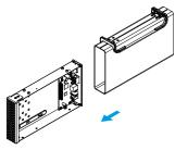
b) Install the hard drive, connect the SATA and power cable and then mount the drive with the four screws from the bottom.
