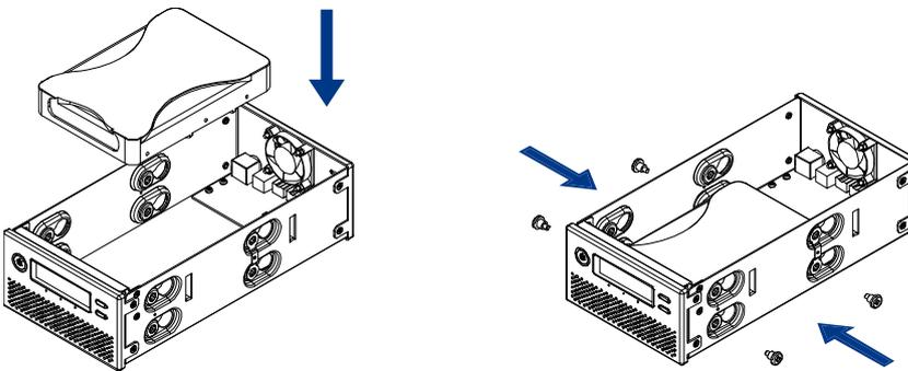
3. Install the second hard drive and mount it with two screws on each side.
