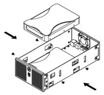
5. Connect the SATA and power cables to your hard drives. Be careful not to damage any components and confirm that the cables are connected firmly.
