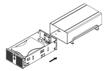
7. Fasten the four screws to finish the assembly.
