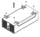
2. Push the inner enclosure out, and remove the outer chassis.
