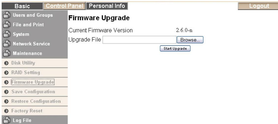
*Note: Never turn off your unit during the firmware upgrade procedure. This may damage your device! If for any reasons (e.g. power supply failure during firmware update) the procedure fails, you may not be able to operate your device any more.*
