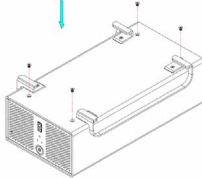
8. Slide the inner enclosure back into the outer chassis.
