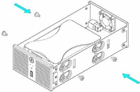
9. Fasten the four screws to finish the assembly.
