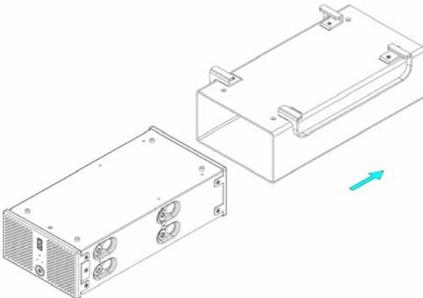
3. Install the first hard drive by placing it in the enclosure and connecting the SATA plus power cables.
