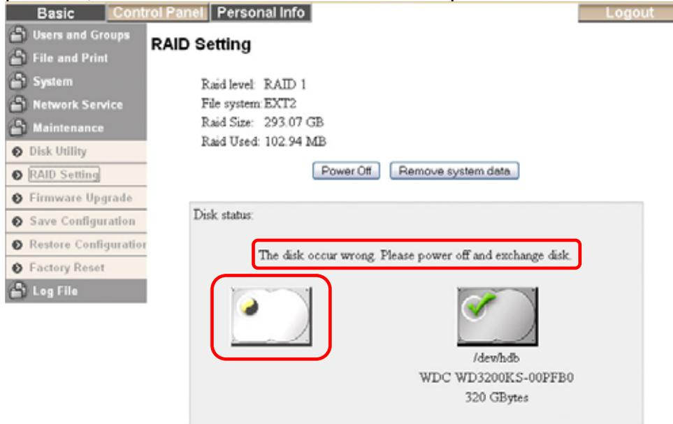
2. Turn off the power, remove the power supply from the wall socket and replace the defective HDD with a new one.
