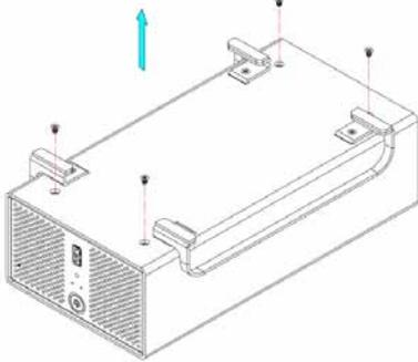
2. Push the inner enclosure out, and remove the outer chassis.
