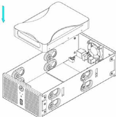
4. Mount the drive with two screws on each side.
