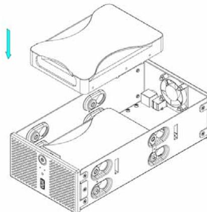
7. Mount the drive with two screws on each side.
