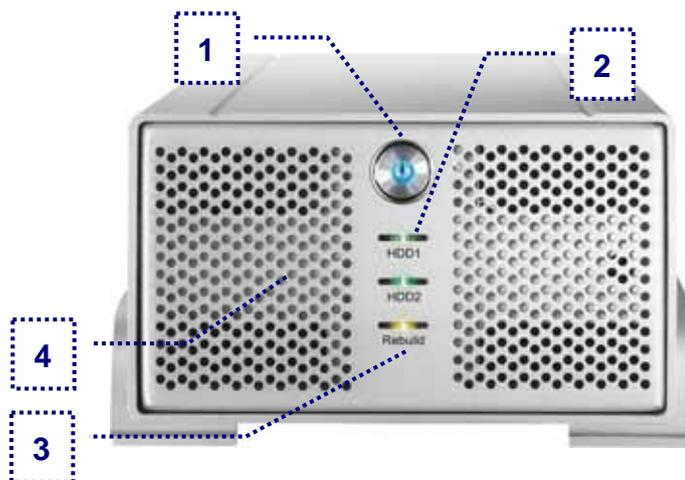
*Note: To turn on the power, press the ON/OFF switch for 1 second and release it. To turn it off, press the ON/OFF switch, hold it for 5 seconds and then release it again.*
