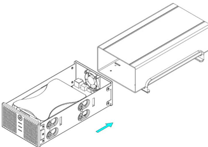
8. Fasten the four screws to finish the assembly.
