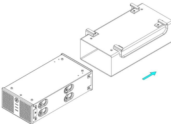
3. Install the first hard drive and mount it with two screws on each side.
