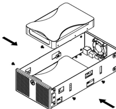
5. Connect the SATA and power cables to your hard drives. Be careful not to damage any components and confirm that the cables are connected firmly.
